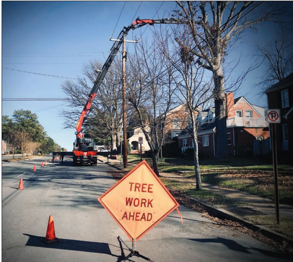
"Large companies use me for trees they don't want to put a climber in or jobs where it would be much more efficient just to use the grapple saw due to site conditions," says the author.
